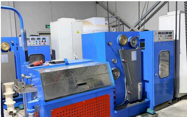
Copper wire drawing line
